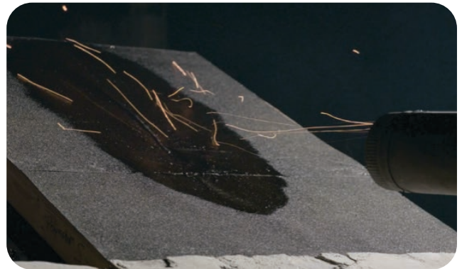
Polyanchor® XFR was exposed to burning embers and 1200°F blowing heat without igniting the wood roof decking.
