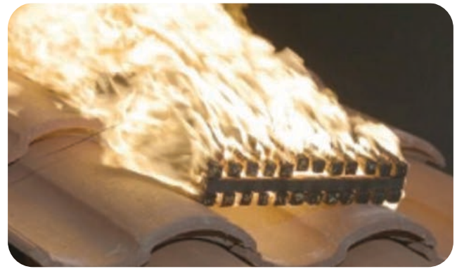
Polyanchor® XFR passed ASTM E108 Class A burning brand test under tile.
