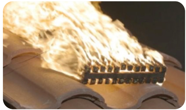
Polyanchor® XFR passed ASTM E108 Class A burning brand test under tile.
