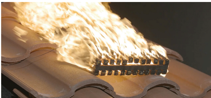
Polyanchor XFR passed ASTM E108 Class A burning brand test under tile.
