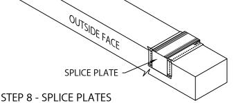
PLACE SPLICE PLATE ONTO ANCHOR CLIPS AT SPLICE JOINTS, 12'-0" O.C. NOTE: REMOVE RELEASE PAPER FROM SEALANT STRIPS.
