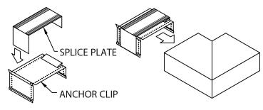
STEP 2 - MITER SPLICE PLATES & ANCHOR CLIPS
