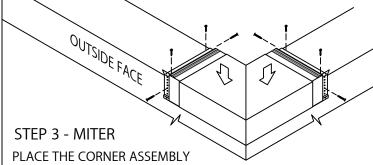
INTO POSITION AND SECURE AT THE EXPOSED EDGE OF THE ANCHOR CLIPS AS PER DETAIL A.
