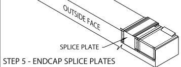
REMOVE RELEASE PAPER FROM SPLICE PLATE
