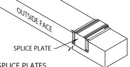
STEP 8 - SPLICE PLATES PLACE SPLICE PLATE ONTO ANCHOR CLIPS AT SPLICE JOINTS
