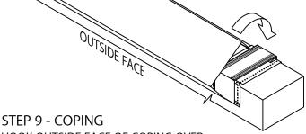
HOOK OUTSIDE FACE OF COPING OVER THE ANCHOR CLIPS AND ROTATE INTO PLACE. ENGAGE REAR LEG ONTO ANCHOR CLIPS BY PRESSING DOWNWARD UNTIL SNAP LOCK OCCURS.
