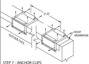
LOCATE OVER ROOFING MEMBRANE
