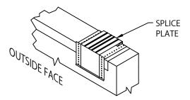
STEP 8 - SPLICE PLATES PLACE SPLICE PLATE ONTO ANCHOR CLIPS AT SPLICE JOINTS, 12'-0" O.C.
