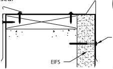
If using an EIFS system, fasten through face w/ fastener of proper length to penetrate through EIFS and attach into structural component
