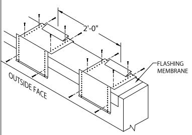
STEP 7 - ANCHOR CLIPS LOCATE AND FASTEN GALVANIZED ANCHOR CLIPS TO WALL AT 2'-0" CENTERS WITH PROVIDED FASTENERS FOR SUBSTRATE (SEE DETAIL A).
