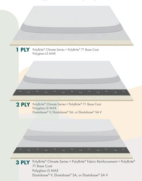
Substrates: Approved High-Density Insulation, OSB, Plywood
