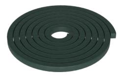
Mapestrip 25B is a sodium bentonite based hydrophilic rubber strip specially designed to form watertight construction joints. The sodium bentonite swells when it encounters water to seal against leaks. Mapestrip 25B is ideal for variety of applications, including horizontal and vertical construction joints, through wall and slab penetrations, and transitions.
