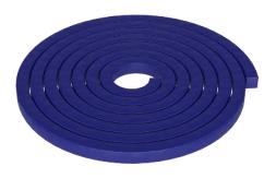
Mapestrip 25 is a pre-formed hydrophilic rubber strip, with an acrylic polymer base specially designed to form watertight construction joints. Controlled volumetric expansion reduces the risk of concrete spalling. Mapestrip 25 is ideal for horizontal and vertical construction joints and penetrations though slabs and walls.
