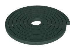
Mapestrip 25B is a sodium bentonite based hydrophilic rubber strip specially designed to form watertight construction joints. The sodium bentonite swells when it encounters water to seal against leaks. Mapestrip 25B is ideal for variety of applications, including horizontal and vertical construction joints, through wall and slab penetrations, and transitions.
