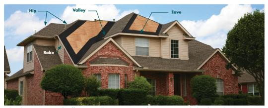
Polystick IR-Xe is especially effective in valleys, eaves, around penetrations, and other demanding locations.
