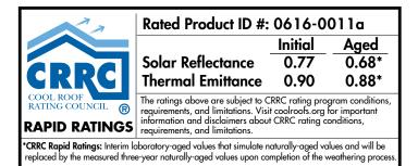
Solar Reflectance Index (SRI) Initial: 96 Weathered: 83
