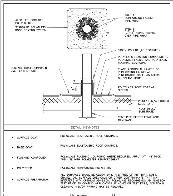
TYP. VENT PIPE FLASHING DETAIL
