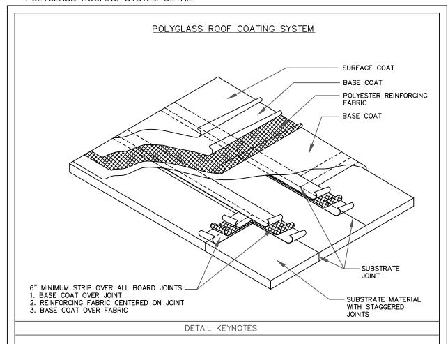
POLYGLASS ELASTOMERIC ROOF COATINGS. SURFACE COAT
